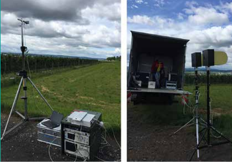
Emulator of the coastal radar transmitter (left) and the two antennas of the passive radar that will be mounted on the drones in the long term (right).
